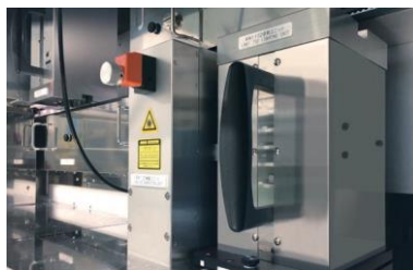
Face/side lighting unit and 3D inspection
