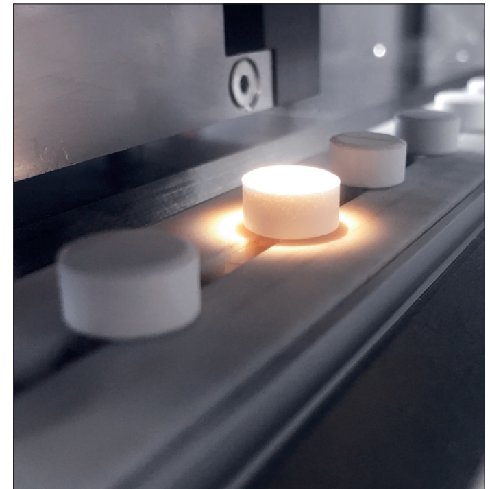
NIR-SRS multipoint tablet illumination
