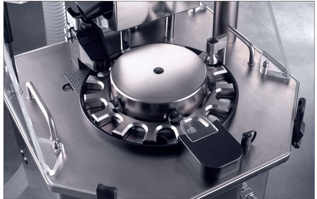
4-Parameter IPC tester (weight - thickness - diameter - hardness)
